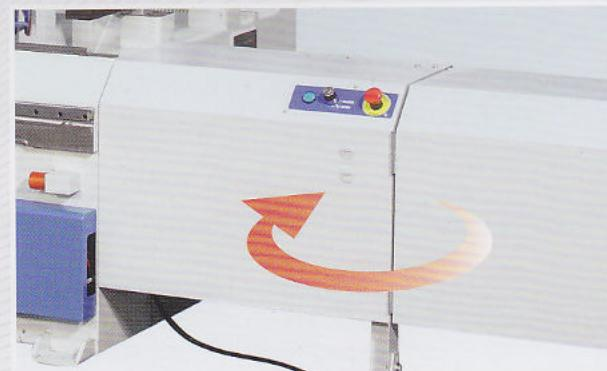
NC controlled centralized automatic lubrication to all movable parts of the machine.
