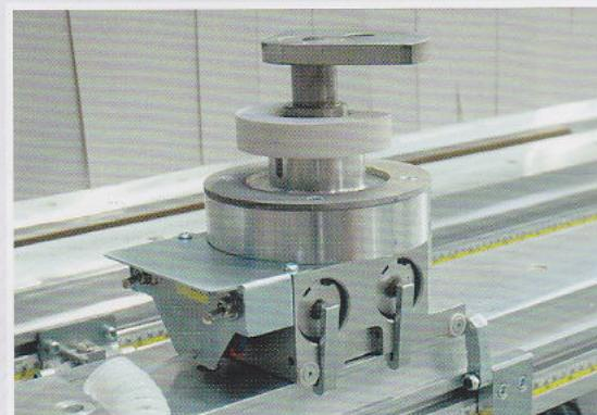
Mechanical clamping systems for solid wood, linear and arched components machining.
