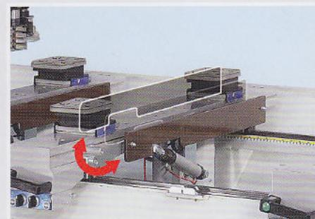
Panel lifting blades for easy positioning of heavy workpieces.
