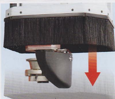
NC controlled adjustable height suction hood (std.) and chips conveyors (opt.) to optimise the suction system.
