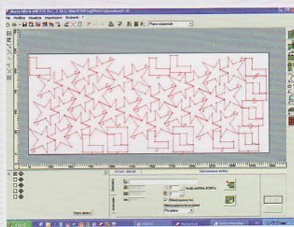
Software package for the automatic optimisation of the positioning of components to be machined on a single panel.
