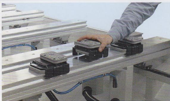
The vacuum locking of the cups reduces significantly the setting time of the working table.
