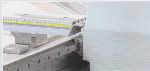
Movement on linear guides of high quality and precision. Brushless motorizations and linear guides with high quality and precision lead bearings for all axis displacements.
