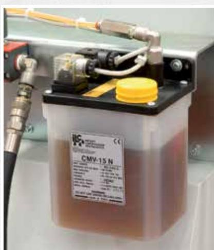
NC controlled centralized automatic lubrication to all movable parts of the machine.
