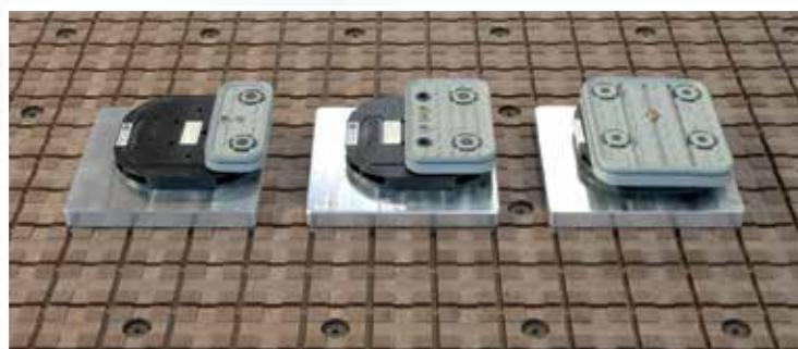
Piece locking also with vacuum cups to be positioned according to the machining requirement.
