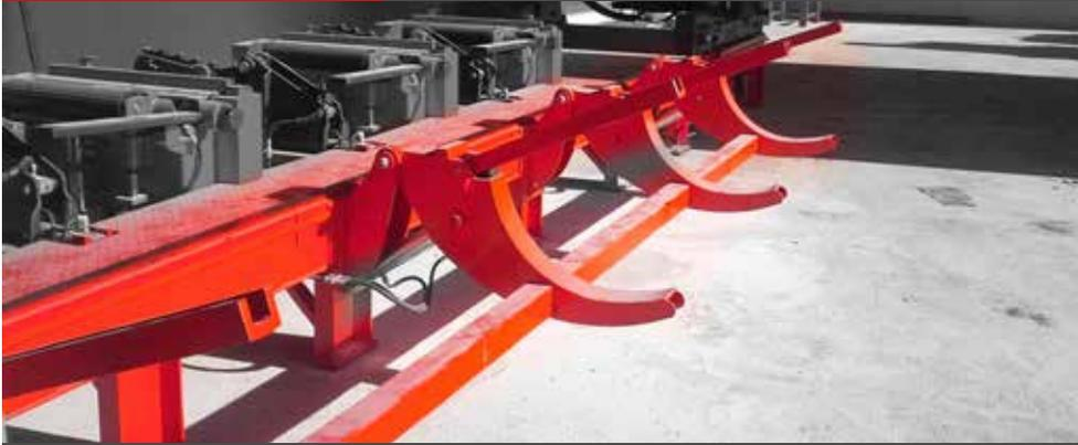
Self loading arms are recommended for middle to small sized bandsaws, with lower capacity of manipulated logs.
