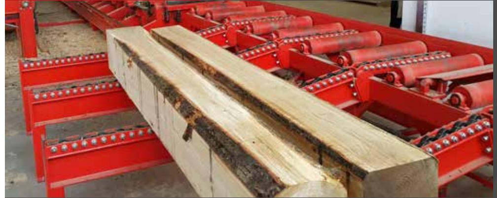
Is located in front of the band saw, where prisms move automatically to side transversal conveyor.
