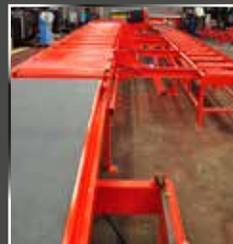
Robust outfeed conveyor for boards works in automatic mode with sorting left/ right or straight.
