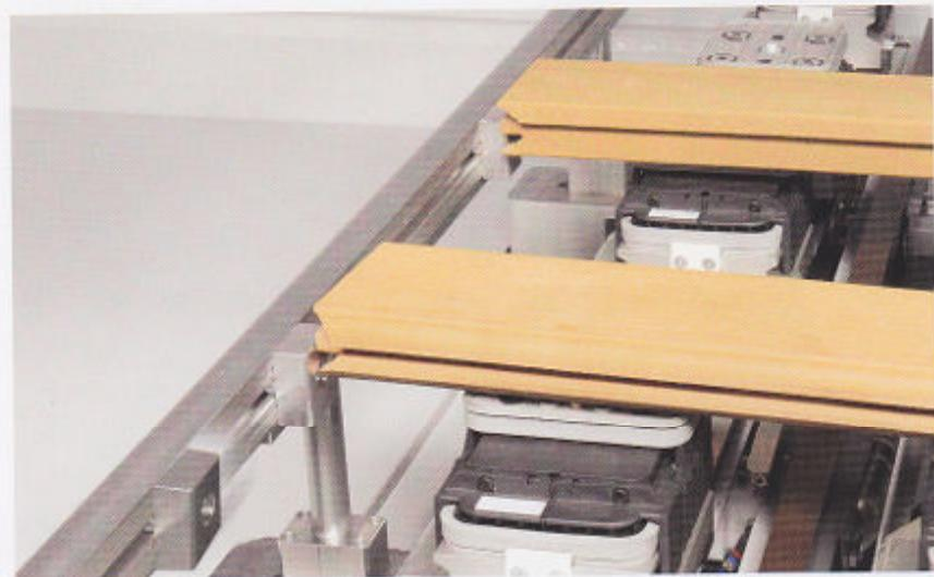
Thanks to the side sliding stops you can position multiple pieces with high precision and without waste of time.
