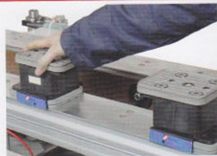
The vacuum locking of the cups reduces significantly the setting time of the working table.
