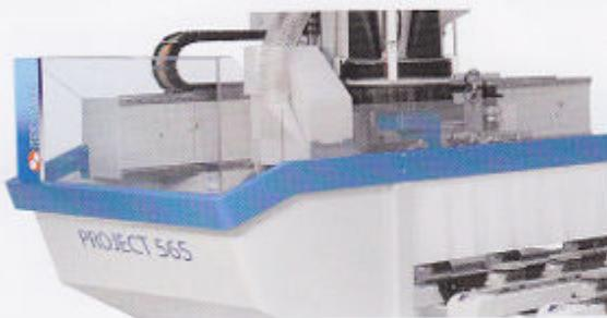
Workings are always controlled by the operator thanks to the transparent total enclosure protection of the operating unit.
