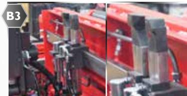
grip with two cylinders + hydraulic lifting of grip pins
